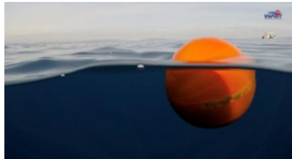
Figure 7. A WAVY drifter floating at the ocean surface. Source: bluewisemarine.ie
