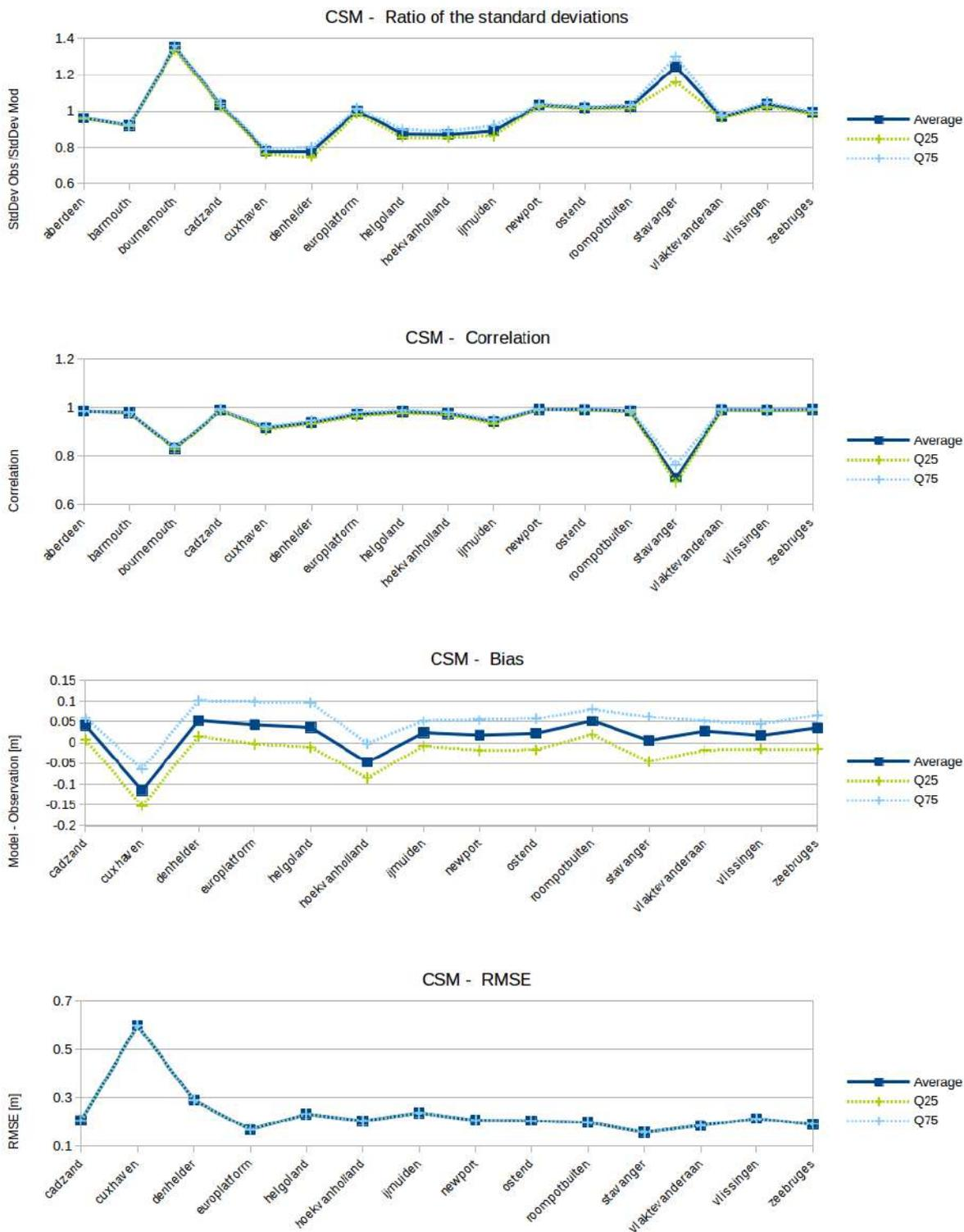
Figure 4.3 Summary statistics of validation metrics per stations, comparing the sea level CSM forecasts to observations. The stations Aberdeen, Barmouth and Bournemouth have only three data points, and are removed from the two last graphs since they strongly deviate from other points.
